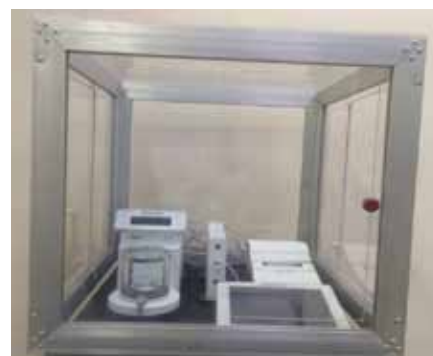
Figure 3.1.2 – Ultra Micro Balance instrument installed at NDTL
