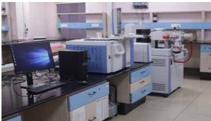
Figure 3.1.1 – New GC/C/IRMS installed at NDTL
